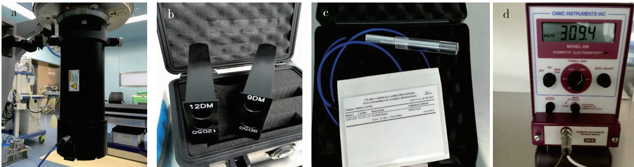
图 1 质控设备 Figure 1. Quality Control Equipment a: Quality assurance applicator; b: Quality assurance phantom; c: Ionization Chamber; d: Electrometer.
